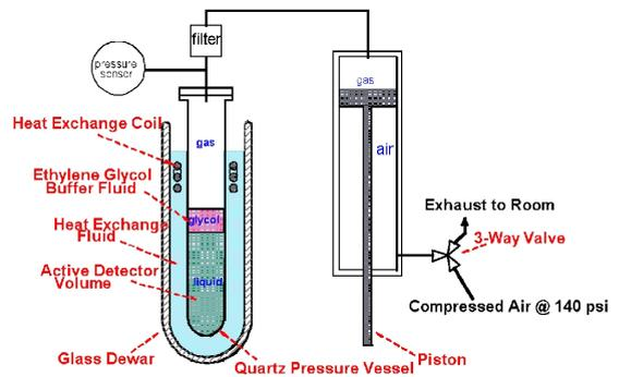
Figure 1. Small Prototype Bubble Chamber.
