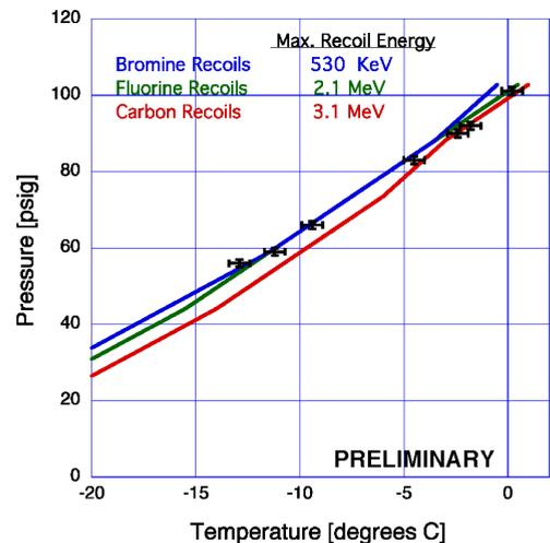
Figure 3. Measurement of bubble nucleation pressure threshold, as a function of temperature, with a Am-Be neutron source. Solid lines show predictions calculated using the Seitz bubble nucleation theory.
