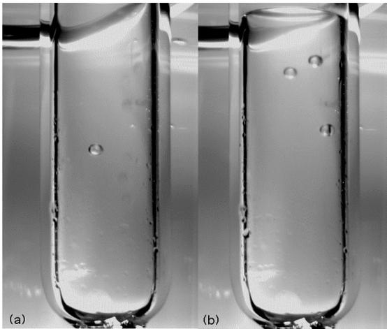
Figure 2. (a) a single bubble produced by exposure to neutrons from an Am-Be source, (b) a triplet of bubbles produced by multiple scattering by an environmental neutron.
